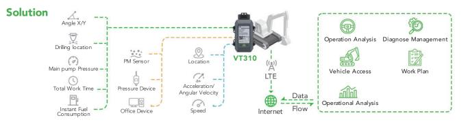
The intelligent solution for heavy-duty vehicle connectivity includes components such as lower-end devices, VT310 vehicle telematics gateway, and remote management platform. The VT310 connects to devices such as pressure sensors and vehicle controllers.
