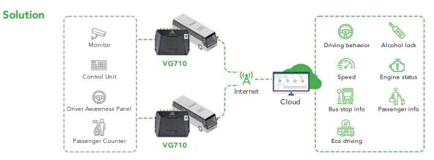
The VG710 connects a wide range of applications on board, including the monitor, control unit, driver awareness panel, passenger counter, etc. Integrating OBD-II and J1939, the VG710 keeps updating the operation status of each bus. With high-precision GNSS and inertial navigation system, the VG710 continuously tracks the bus's location whether GNSS signal is available or not.
