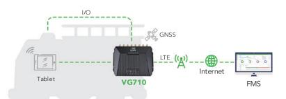
Emergency lights and siren of each firetruck is connected to the VG710 via I/O. The VG710 also offers fast and reliable on-board Wi-Fi to the navigation tablet which helps the driver receive dispatch routes from the management center. Built with 72-channel GNSS, the VG710 keeps locating each firetruck and sends the data back to the fleet management system.
